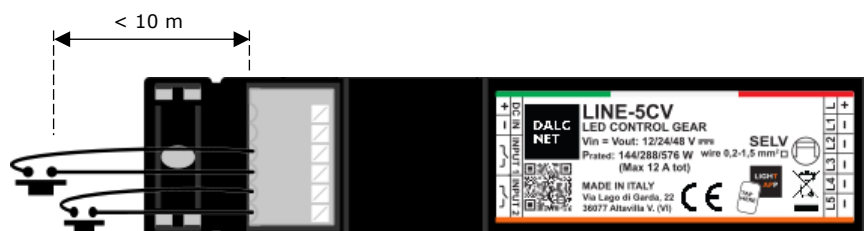
Figure 7: Local Command connection diagram for Short Distances
